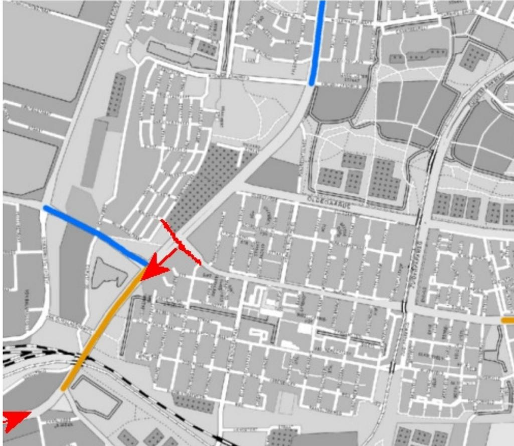
Figure 2: QUADMAP pilot area Groene Kruisweg; blue marked road will have low noise pavement in 2013 and orange marked roads were repaved in 2011 and 2012
